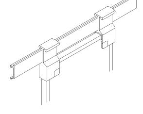
With the corner track mounts and track bumpers installed, place the EganBoard onto the EganSystem T rack.
